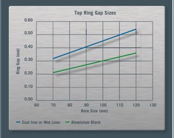
For higher running temperatures such as supercharging, use an additional 0.005 mm per 10 mm of bore size, and for very high temperature operations such as drag racing an additional 0.007 mm per 10 mm of bore size.
